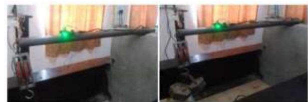
Figure 5 Composite blade in unloading and loading condition
